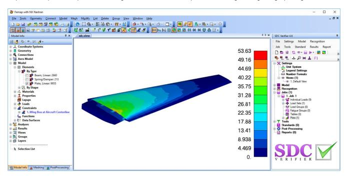
The complete verification procedure of the structure is stored. When the design is modified it requires only one-click on "Regenerate" to rerun all the calculations and regenerate the report.
