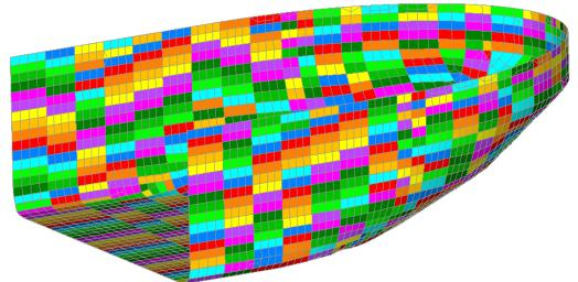
Recognition is based on mesh connectivity and can be performed on any structure build using plate (shell) elements:
