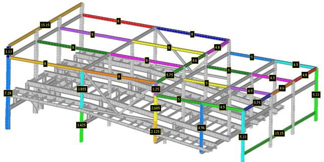
Buckling length is calculated between the Joints and does not depend on the model mesh.
