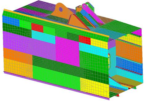
Results can be presented over sections (frames/longitudinals/decks) and results which are above the limit are highlighted with red:
